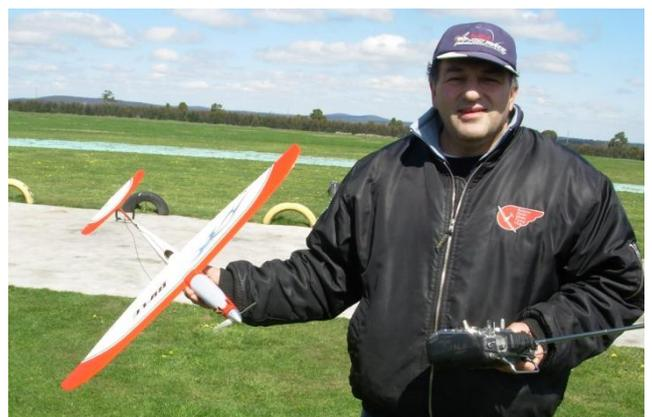
The Rifle is built by Great Planes from fibreglass with a few strands of carbon fibre in the bottom of the wing for extra strength. Aileron-elevator, hand launch and belly landing; it's a slippery little sucker with nothing hanging out. At 31" span and 18oz (785mm, 510g) it is a small, pretty little plane designed to give you a taste for speed, and send you to the optometrist for a new set of glasses.
