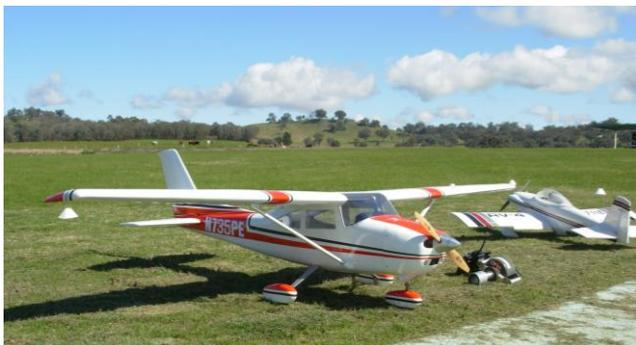
*Anthony Mott's big Cessna 182 (3m wingspan) and powered by an OS Gemini twin cylinder four stroke. Model flew with authority and certainly looked realistic in the air and on the ground. And yes it's an ARF as well.*
