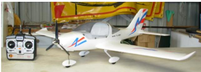
TL 2000 foam electric model complete with geared brushed motor, 4 channel SAPAC radio gear on 36.050MHz. 1150mm wingspan.
