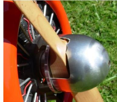
thought it might have been a piece of the plastic dummy motor. After stopping the engine I noticed the spinner had moved on the prop in the direction of rotation and broken away two sections of the spinner cone. The model was taken back to the pits where the cone removed to make sure prop was tight which it was.
