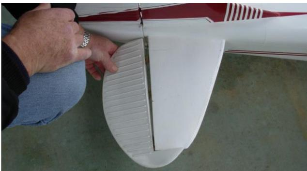
And then we discovered loose elevator hinges – it was time to put the Cessna in the trailer.
