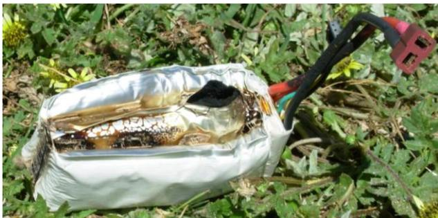
*The battery has burst its seam where it compressed. There is plenty of padding on sides but not in direction of flight.*
