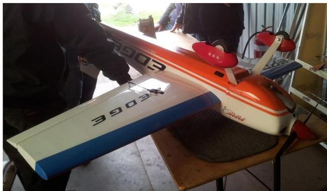
*The Edge is about 72" span and powered by an OS120 2 stroke. The ailerons are large on these aerobic models and therefore impose high load on the servo.*
