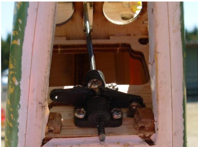
*The plastic arm had broken away from the brass insert which has a set screw to locate on the rudder shaft. This allowed the rudder to flutter as well and prevent controlled movement.*
