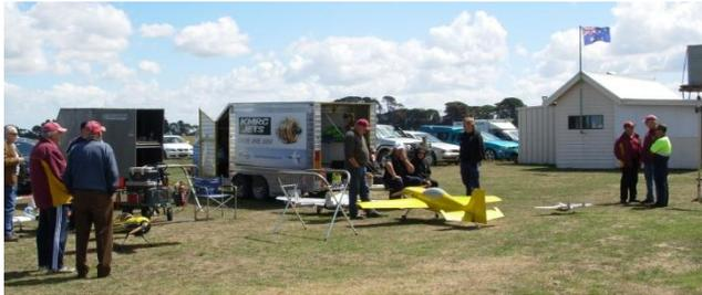
Ken Mollison's big yellow Extra powered by a DLE111. Flew once but suffers from chronic elevator flutter when full power applied. It appears elevator requires static balancing by adding mass to the balance horn.
