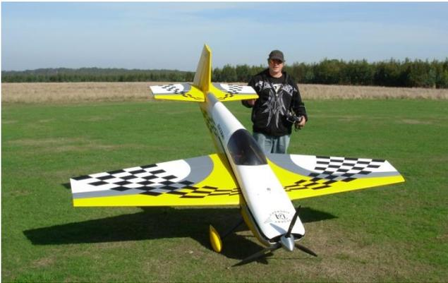
This shot shows just how big the Extra is. 40% scale by Composite ARF and powered by a DLE 170cc twin.
