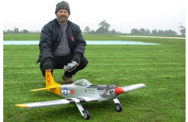
David Filmer can be seen here with his new Hanger 9 PTS (Progressive Trainer System) P51 Mustang Trainer, powered by an Evolution 40 two stroke motor. Model comes with trainer aids: Clear aerofoil sections taped to the leading edge of the outer wing panels, speed brake system on the fixed L/G and two position flaps that can be rigged up to a servo.
