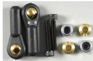
It's a good idea to fit a retaining washer over control surface ball joints to prevent them coming completely adrift should they pop off the ball. If they are a tight fit it is unlikely to happen in flight, but some we have seen can be pushed off and it is better to be safe than sorry.
