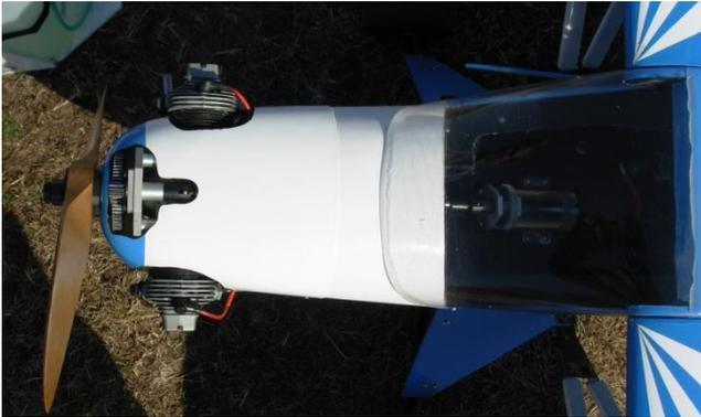
Note the onboard electric starter mechanism.
