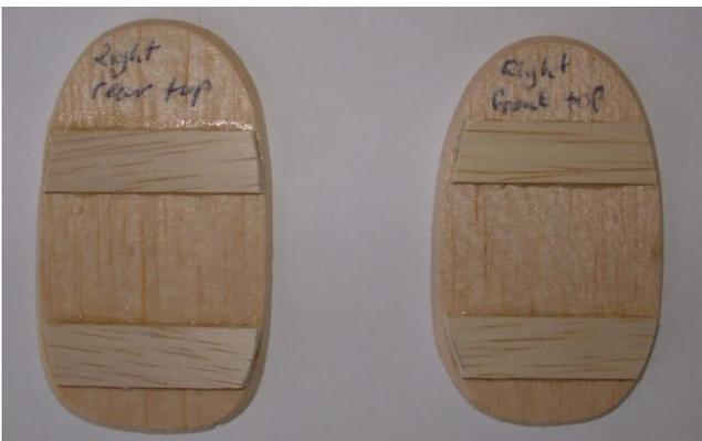
The drawing was then printed and the four (two the same) formers cut out from the sheet as a rectangle and stuck to hard 1/8" balsa using 3M spray adhesive then cut out on scroll saw. A chamfer was then sanded on one edge and with very little adjustment they fitted the required location. As you can appreciate with the
