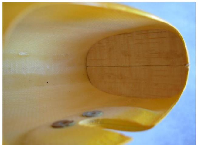
The formers were then epoxied in place along with the extra outer side plate (not shown here) to produce a very strong and hopefully serviceable wheel spat.
