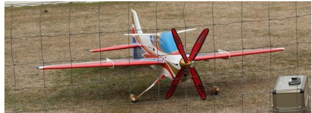
This model has contra rotating props. It's via a single electric motor driving through a gearbox. It definitely has a distinct sound in the air.
