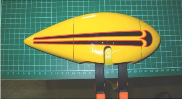
A photograph was taken from each end of the spat with the lens lined up with the centre of the spat to reduce distortion. I had to use an SLR camera instead of compact to get the focus on the line for the rear photo. The compact wanted to focus on the tip making the line blurred.
