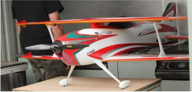
Glenn W. managed a close up shot on Saturday of Glenn Orchard's Citrin while sheltering from a shower in the BBQ area. Note the slots in the carbon fibre spinner to provide cooling for the electric motor etc.
