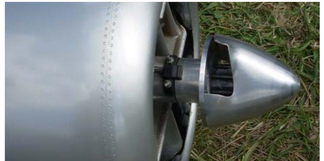
The propeller blades broke off at the hub in flight while the motor kept running – not much thrust though! This is another reminder of why we mustn't stand in line with spinning props.
