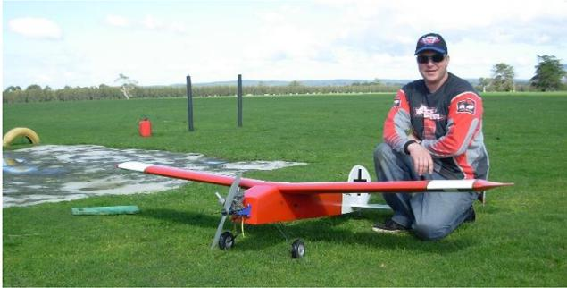
Mat with his latest Graham Waterhouse built Ugly Stik. Model is powered by an NGH 17cc petrol engine and has a wingspan of 2170mm.
