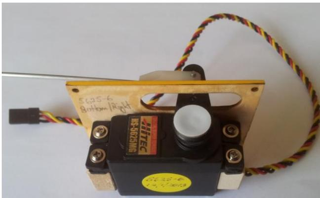
The alternatives are thread locker or a dab of silicone on the screw head and arm, but these are messy to use and can be difficult to undo.
