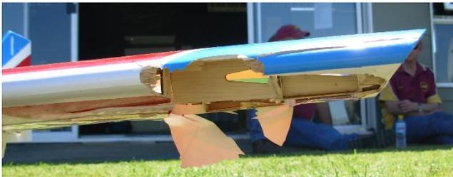
*This is what happens when Scanner wing comes into contact with pylon pole – no damage to pole.*
