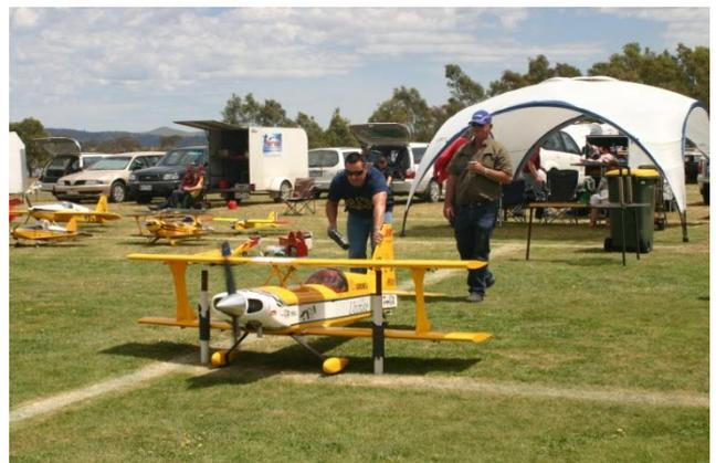
A very large Ultimate Bipe powered by a DA 150cc twin cylinder petrol engine.
