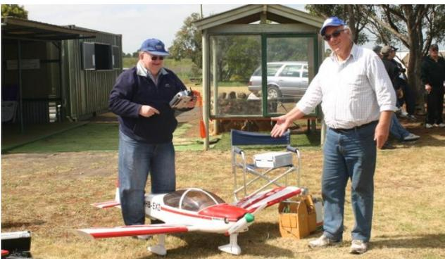
Noel Whitehead with his latest "flying only" model. He was being ably assisted by Cliff McIver to get the motor adjusted and tuned. The model is a Robin 2160 by Austars and is powered by an OS FT 300 50cc twin 4 stroke. It's quite a large model having a wingspan of 2.2m and tipping the scales at 9.1kg.
