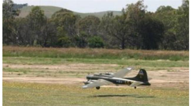
Almost there! By the time it had landed and rolled to a stop, only one motor was running. The problem is the exhaust outlets are fabricated pipes and have no expansion chamber and hence muffler pressure for the fuel tanks. Some modifications will need to be carried out to ensure reliable engines. The model obviously flies very well and all importantly, when it loses motors.
