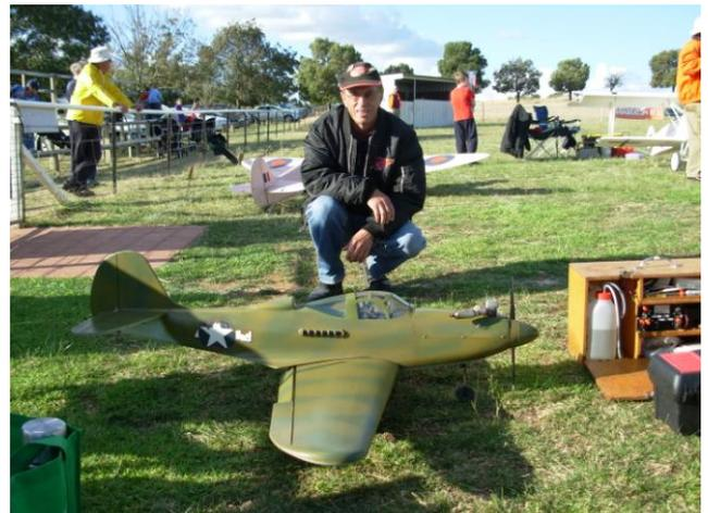
*Roger and his old Top Flite P39 Airacobra – originally powered by a Webra 61 2 stroke in 1976 with Kraft Series 75 radio gear. Now has a Magnum 91FS, JR radio gear, but still uses the original Kraft Multicon retracts with separate 650mAh AAA NiMh battery pack.*
