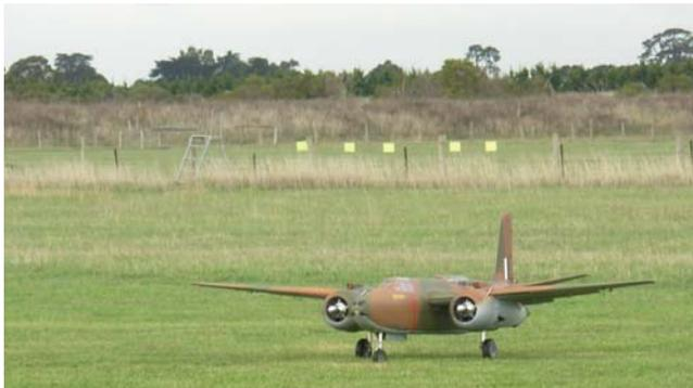
Mike Farnan's WWII Boston powered by two OS Sirius 50cc 5 Cylinder four stroke radial engines. Model is very impressive on the ground and in the air. (Around 3m span)
