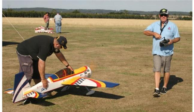
Greg Lepp's ill fated Yak 54. During the second flight (might have been on landing approach going by the scores) it lost radio control and crashed. Apparently the plug lead braiding wore through where it was rubbing on the cowl. The braiding is to shield against radio interference whether 36MHz or 2.4GHz. Rotten luck Greg! Photo was taken while getting ready for first flight. Noel W's Robin less right u/c leg is still on runway in the background.
