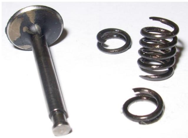
OS91 FS-SII Inlet valve and broken spring. For the record the head is  $\varnothing 11.2\text{mm}$ , stem is  $\varnothing 3\text{mm}$  and 26.4mm long.
