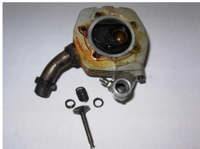
Exhaust valve has also been removed and the carbon deposits cleaned off. I found that an old X-acto blade was an effective tool to scrape the carbon off the valve stem, head and around the seat without fear of scratching.
