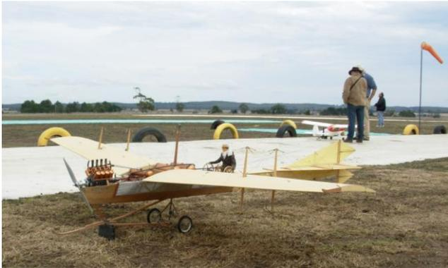
*Murris 92" span Antoinette powered by an electric motor. It was thought the vibration level from an IC engine might be too much for the delicate airframe and would spoil the scale like appearance.*
