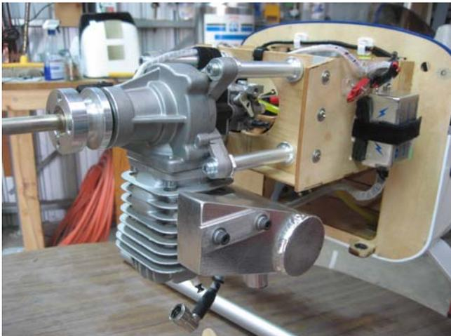
*Under the bonnet! The DL50 and "Pitts" style muffler. (I suspect the load distributing plate under the muffler bolt heads is Matt's finishing touch.)*
