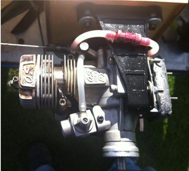
*The old OS91FX; showing catastrophic failure of the crankcase.*
