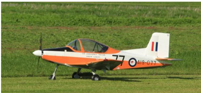
Noel Whitehead's CT4 taxiing out for take-off. Wing span is 2.4m, just under the 15kg weight limit and powered by a Zenoah 80cc twin. Looks great and flies well. 2<sup>nd</sup> Flying Only.
