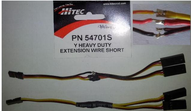
*Inset, you can see the open joint on one of the black leads. With the heat shrink tubing everything looks peachy but beneath one never knows how good the soldered joint is.*
