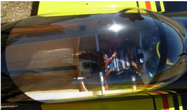
The power board has a magnetic switch mounted to the side of the fuselage enabling the controls to be turned on & off by holding the key over the pickup sensor.
