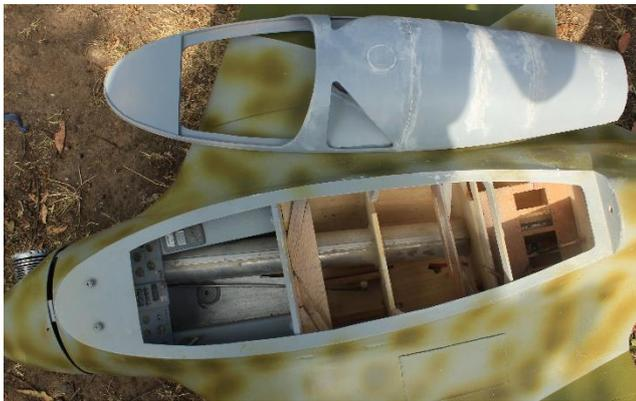
*The Komet is powered by a Webra 120 2 stroke this time instead of the OS 60 Hanno Special. Exhaust exits through the aluminium tube running through the fuselage.*
