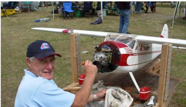
*Glenn wasn't happy with the way the motor was running during the first flight so he decided to take the cowl off and do some maintenance under the watchful eye of Noel. Amongst other things the muffler connection to exhaust port was resealed and yes, the engine cleaned.*
