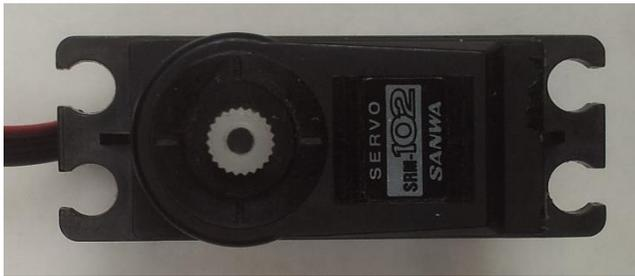
Sanwa servo output shaft is 5.95mm diameter and has 23 teeth like JR.
