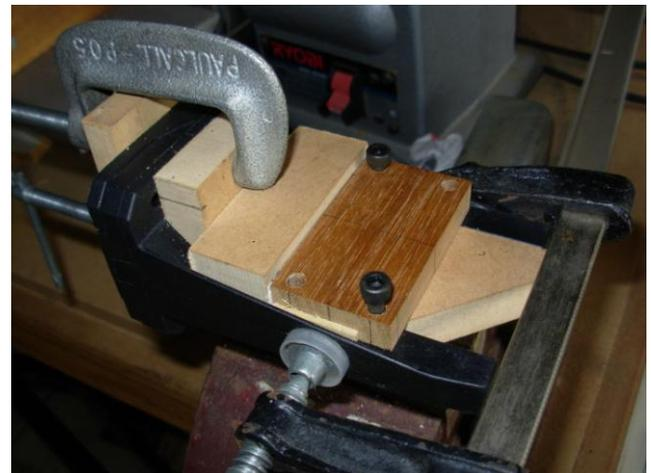
Spacer blocks and drill block were used to drill the four 5mm mounting holes. The spacer blocks were cut to size so as to achieve the correct position for the engine.
