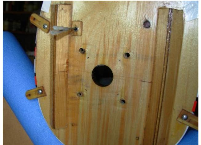
*Original mounting holes were plugged with tight fitting dowel and redrilled using a drill block clamped to the bulkhead through the fuel tank neck locating hole.*
