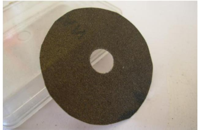
*Friction disc made from 220 grit carborundum paper. The 40mm diameter disc was needed to prevent prop slipping on a spacer washer.*
