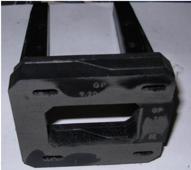
*Mounting surface has been faced off carefully on bench belt sander. It is surprising how uneven they are! 100% contact isn't necessary but it needs to be around the mounting holes.*
