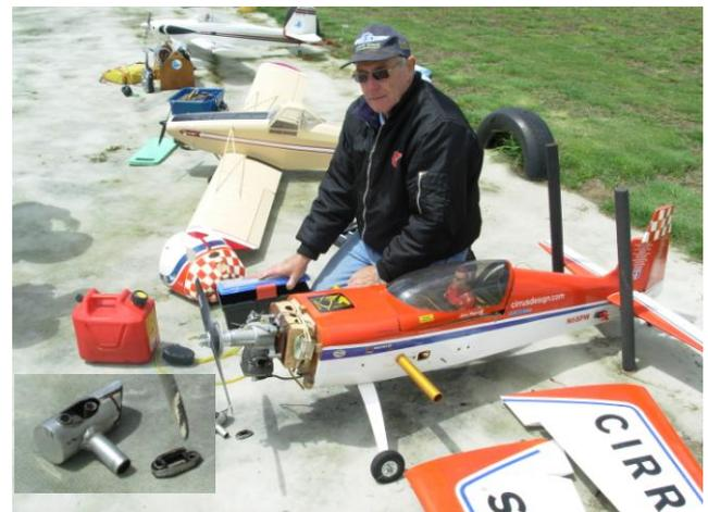
S@#% happens Glenn! The muffler cracked and broke off the 3MM 53cc petrol motor during round one. Keeping the muffler tight has been a challenge with this model.
