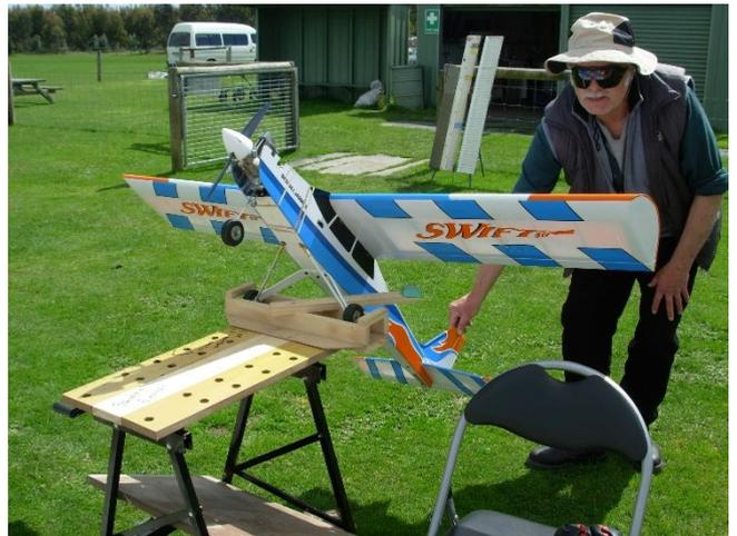
Len scoffed at ARF's however he did succumb to investing in one or two – always with extensive modifications. He fabricated this frame which was clamped in a work bench stand to support the Swift ARF while starting. Saved having to bend down all the time. Enabled the nose to be elevated to ensure the engine tuning was just right.
