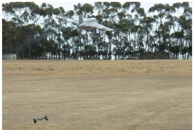
The Komet gets aloft with the dolly dropping away. You can see the elevon control deflection in the photo. Lots of left being applied here. It's all happenings on take-off that's for sure. The trees in the background are on the northern boundary and are a long way from the flight line. The worst thing is when landing from the north your model tends to get camouflaged making it difficult to see under some light conditions.
