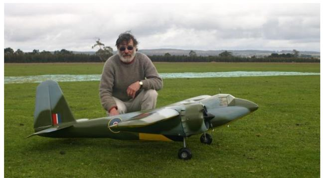
*John with his latest model off the 'assembly line'. This one's a Miles M.33 Monitor which was designed to tow gunnery targets.*
