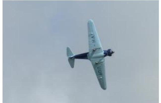
*Just managed to get this shot on one of Mat's many passes over the field. You can see the wheels retracted back into the wing although half of the wheel remains exposed as did the full size.*
