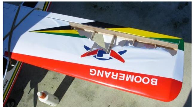
*The covering tore away on the upper and lower surfaces of the left wing during the first flight. Very unusual!!!*
