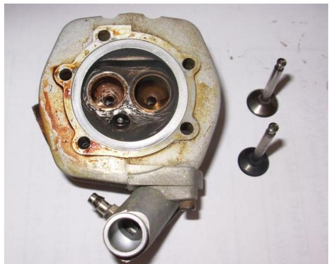
Once all the carbon was removed it was time for reassembly. The tricky part is fitting the tiny valve retaining collets. Extreme care must be taken because if
