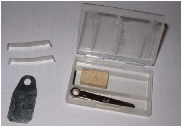
*Valve spring compression tool (lower left) fabricated to fit valve retaining collets together with OS valve clearance adjusting kit. (Came with OS120FS 12 years ago.)*
