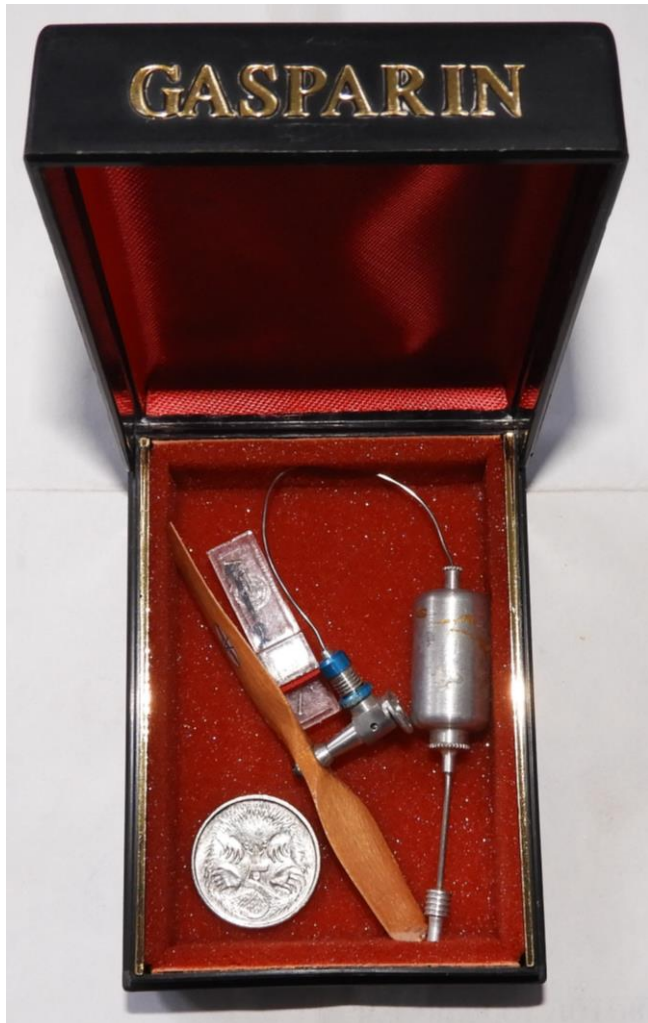
Photo of Murri's Gasparin CO 2 G6 motor with 5c coin to show off its diminutive size. Has a bore & stroke of 2mm, giving it a capacity of 6.28mm 3 . Weighs in at 3.6g and is rated to power a 200-330mm wingspan model weighing 4-6g.
