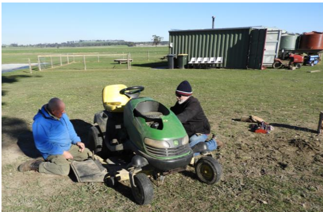
Wire cable got tangled up around the blades of the John Deere making it a good time to drop the deck, remove the wire and also cleanout the caked on grass & dirt.
