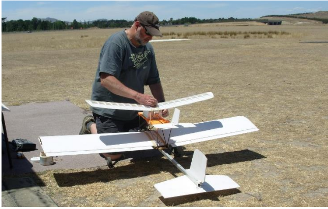
Greg Savage with another of his core flute constructed models. This one has a glider to take up and release. (Sunday 17 th January)
