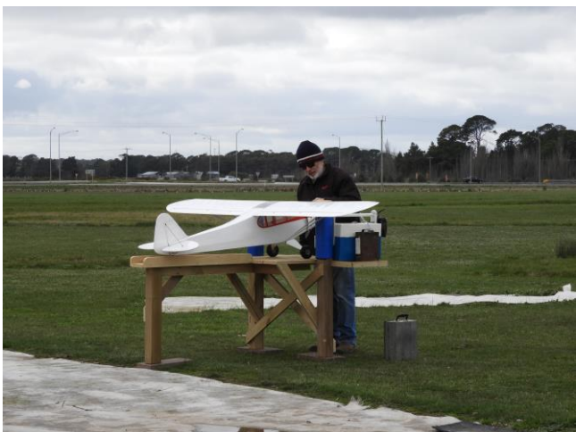
Peter Evans also tried out the new stands with his Cub. You need to be very careful, particularly with large models, lifting off the stand with the engine running. Lift from behind to make sure you don't get tangled up with the prop.
