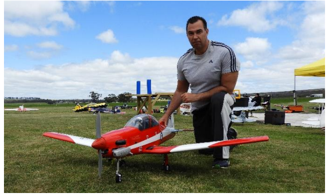
Anthony Mepstead with his new Blackhawk PC-9. 1800mm wingspan with OSGT22 petrol power plant.
