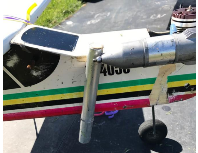
Nick's custom exhaust extension to deflect that messy oil away from the airframe.
