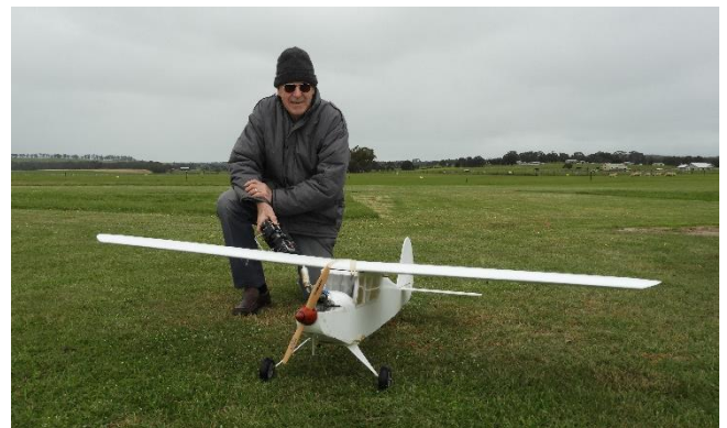
Jeff Dowsley with his scratch built LA Special powered by an OS 52 four stroke engine.
