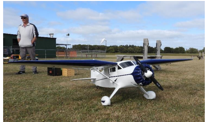
Robert Lauder's Stinson Reliant built from the Top Flite kit. Model is powered by the OS 40cc petrol four stroke and has a wingspan of 100.5" or 2.55m.
