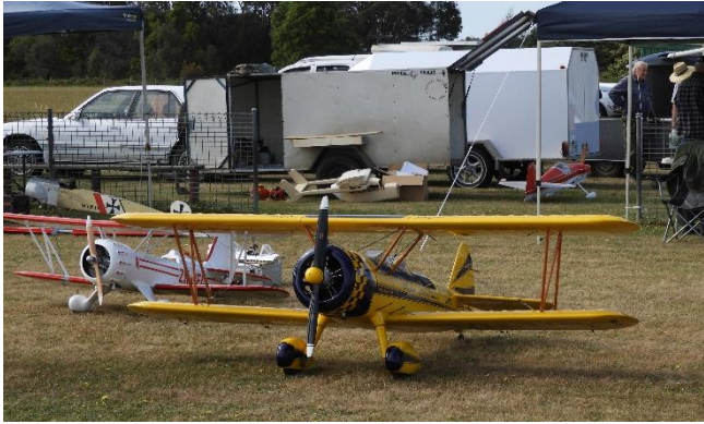
215cc Moki 5 cylinder radial powered 1/8 scale Super Stearman built from a Balsa USA kit.
