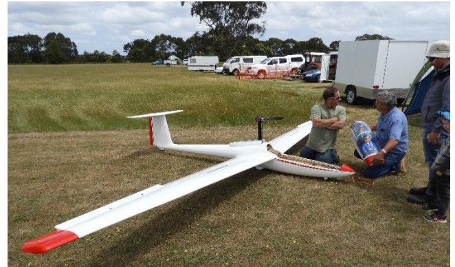
The Phoenix Models kit of an ASK-21 glider. 6.5m wingspan and weighs around 25kg (I think that's the weight mentioned).
