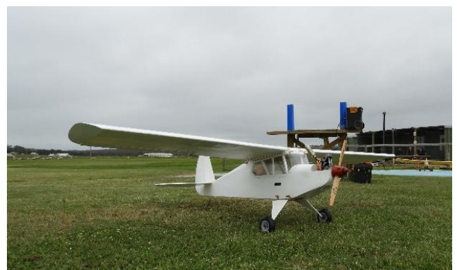
Another shot of the LA which is covered in tissue and doped the way model aircraft were traditionally built.
