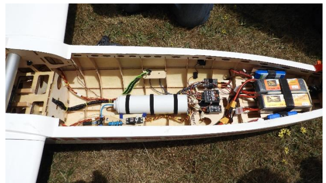
Batteries in the nose and cylinder to store compressed air to raise the power pod
