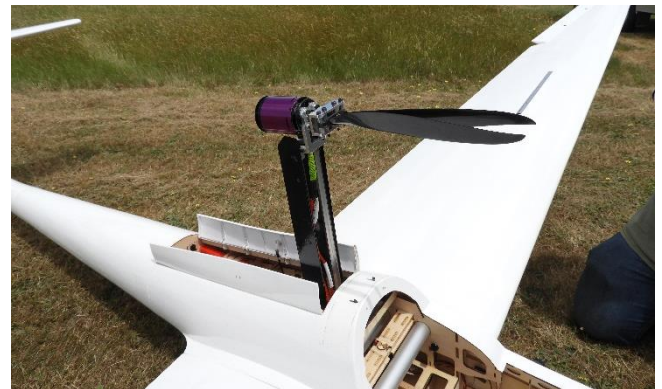
The retractable power pod which is raised & lowered pneumatically. The electric motor is a Hacker 60.
