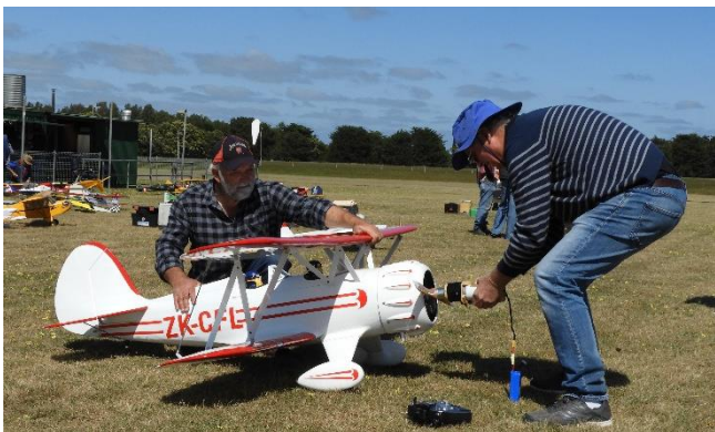
Barry Angus from Mildura starting the twin cylinder petrol engine in the Phoenix Models WACO YMF-5.
