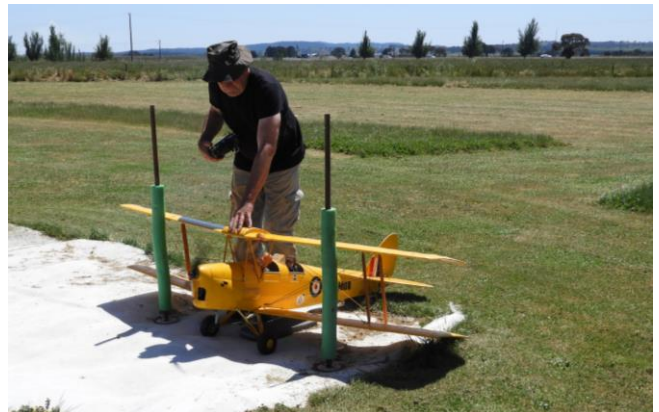
Sunday 12 th November, all systems go – the old OS FS-120S II sounded like it was running well, Graham must have done a good job cleaning it out.
