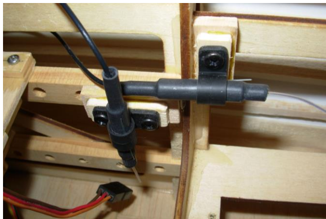
A short length of fishing line provided sufficient interference to prevent the BODA aerials sliding out of the rubber mount. Don't know why they were loose on these two receivers, they weren't on the previous two – must be the weather.
