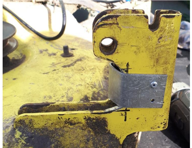
The back of the deck belt has been hitting the support bracket. It's been ground at an angle parallel to the belt path and a plate wrapped around & riveted into place.
