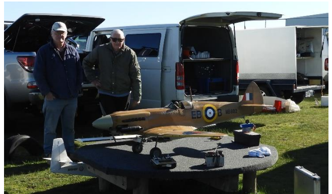
We had the Spitty on the table to check the balance upside down then right way up in flying attitude. We determined it needs about 350g in the nose.
