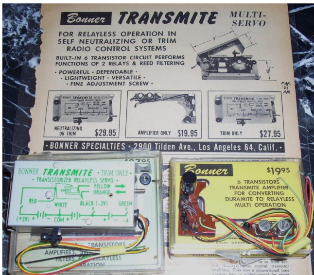
These were the Bonner Transmite servos that came as either trim or neutralizing types. Throttle used trim type while control surfaces used the neutralizing type.
