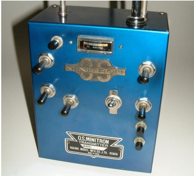
An OS Minitron 12 channel transmitter which dates back to at least the early 1960's. A far cry from today's computerized sets.
