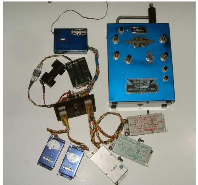
OS Minitron 12 Channel Reed set. How would you like to mount all this gear in your model today? Those Bonner Transmite servos were huge. A set sold on eBay in the UK in 2011 for £370. I wish I still had mine!!!
