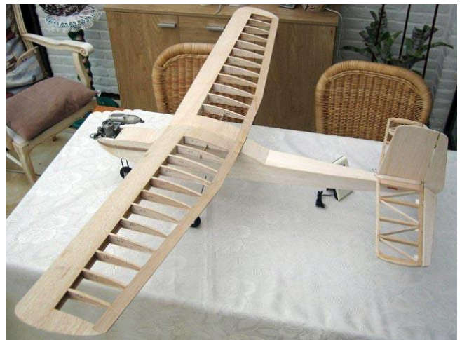
The wings and tail assembly (vertical & horizontal stabilizer) were both held on by rubber bands which allowed for the inevitable mishaps while learning. It was cleverly designed with the wooden engine bearers protruding externally for extra strength without bulking up the fuselage cross section.
