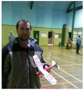
Dan Missen of Ballarat Aero Modellers holding his Flyzone Tiger Moth. 15" wing span and foam construction, ready to fly out of the box. Weighs in at a miserly 33g.
