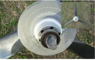
Close up shot showing the fractured crankshaft of the DLE170. The texture along the break suggests the crack has been growing for some time. Highlights the stress created swinging a 32" diameter propeller particularly when the aircraft is doing high G manoeuvres.
