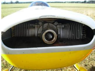
The crankshaft broke and pulled away cleanly from the engine and airframe without causing any further damage.
