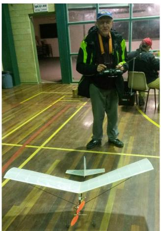
Kevin Howard also of Ballarat Aero Modellers with his ERat - looks like about to take-off. 1.2m wing span, weighs 180g, and is fitted with a 600mAh battery & brushless motor.
