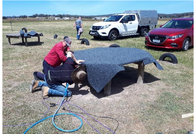
Alan had his pneumatic staple gun to secure the carpet underneath then trimmed off the excess. The carpet will also help to hold them together.
