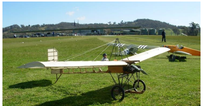
Ken Osborne's Robbins Monoplane (aka the Albury Flyer). Powered by an OS60FS engine.
