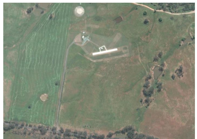
The main runway is predominantly E/W and 130m of it is concrete 10m wide with grass sections at either end. You can also take-off & land on the grassed runway on the other side (south side) which many did.
