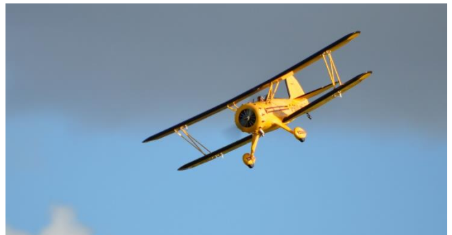
Roger Carrigg's Great Planes WACO YMF-5 powered by an OS155Alpha four stroke. I've had bounce problems on landing ever since its first flight but after replacing the foam wheels with Dubro 3.75" pump up wheels the tendency to bounce has been mitigated significantly. I had the same problem with the Super Stearman and found the better wheels make a remarkable difference.
