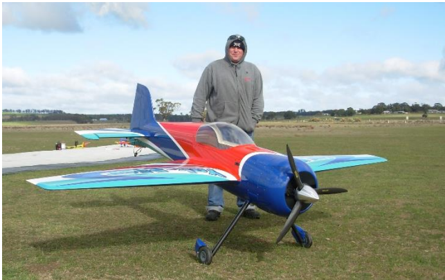
Mat's new Yak-55sp which he test flew on Sunday 2 nd August. Powered by a DLE170 turning a 25.5"x12.5" carbon fibre 3 blade propeller.
