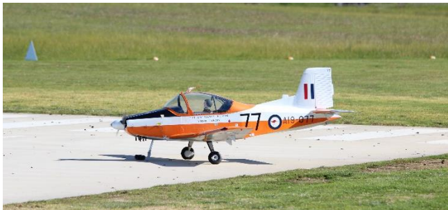
Just as the CT4 turned onto the runway for take-off for the 2 nd flight the nose and port main wheel hubs collapsed.
