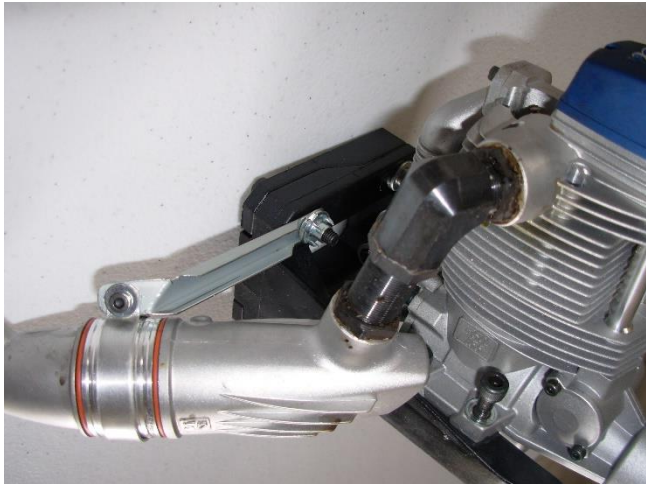
Muffler bracket fabricated from a section cut out of an old printer chassis.
