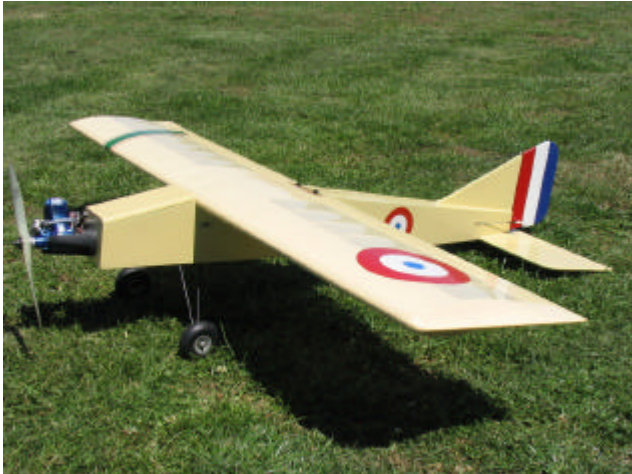
Graham Waterhouse had his latest creation out at the field on Sunday 13 th February and gave it a test fly after the Roy Gladman competition. Model flew superbly and we recommend that any new modeler should look at the quality of the paint work. You can't pick it from the film on the wings. This was accomplished with tissue, talc and dope.
