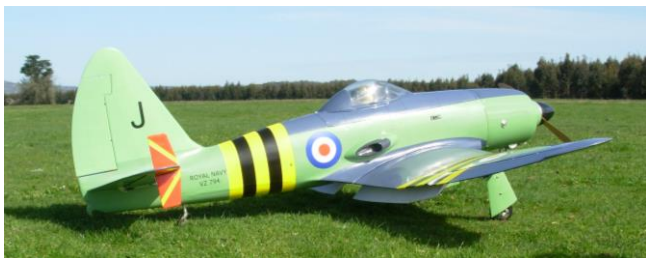
Wayne Goodwin’s Westland Wyvern. The Wyvern began as a Westland project for a naval strike fighter, with the engine (a Rolls Royce Eagle piston engine) located behind the pilot, driving a propeller in the nose via a long shaft that passed under the cockpit floor. This was abandoned for the production models which had a conventional nose mounted turboprop driving contra rotating propellers.
