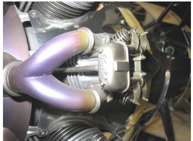
How's that for attention to detail! The rocker covers are engraved with the word Bristol and the exhaust stacks are painted to show heat effect. Looks so real!
