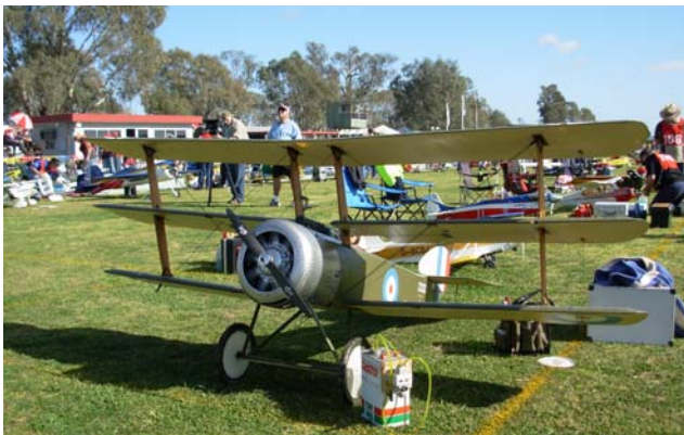
Robert Zyp's 1/3 scale Sopwith Triplane. The fuselage folds through the roundel for easy transportation and flight setup. Model won pilot's choice.
