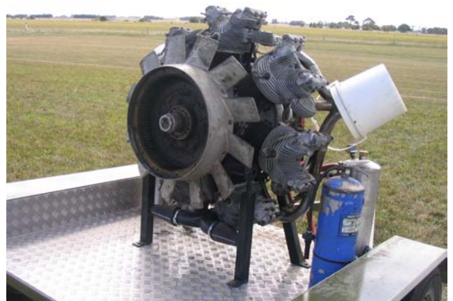
It's a small radial engine out of a WW2 Stuart tank. The owner ran it a few times throughout the day.
